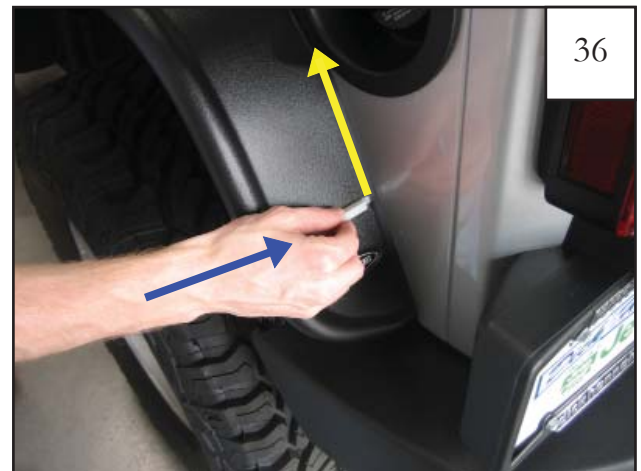
Starting at one end, use the flat edge of the supplied edge trim tool to further adhere the edge trim to the vehicle surface. Slide the tool along the edge trim while pressing it in toward the vehicle surface.
