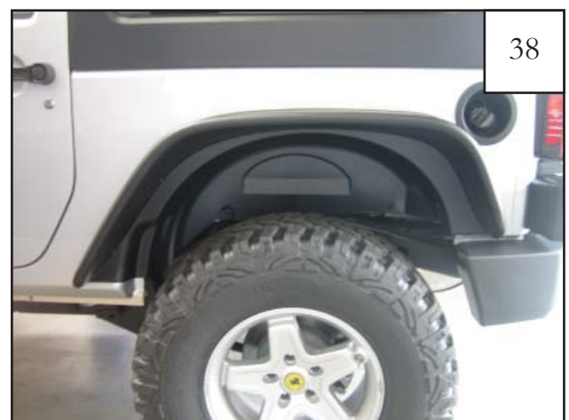
Completed rear driver's side flare installation.
