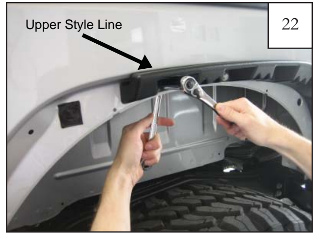
Step 4 Using a 1/2" socket wrench and a 1/2" wrench, tighten all bolts until inner piece is snug against fender. Do not overtighten: see step 23. Inner piece should rest along upper style line of sheet metal radius and not below it: see step 18.
