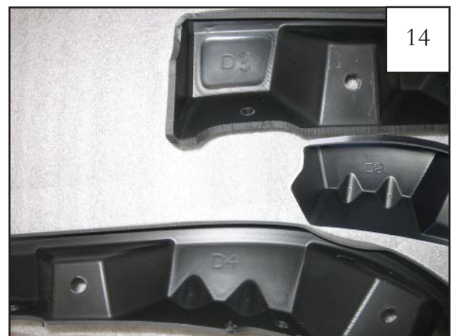
Locate the flat flare rear inner pieces. The driver side rear inner pieces are marked D3, D4 & D8. The passenger side front inner pieces are marked P3, P4 & P8.
