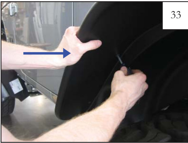
After all screws have been started, tighten the pan head screws by firmly pressing the flare toward the vehicle while tightening.
