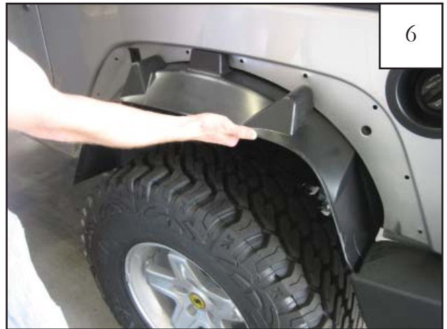
Hold the splash shield in place using supplied 1/4" Panel Retainers through factory holes halfway. Do not fully install Retainers, leave them half out. They are only used to hold splash shield in place for marking. See step 24 for locations.
