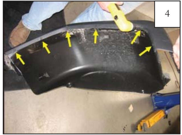
Use a drill with a 5/16" bit to drill through six plastic rivets along edge of flare/splash shield. Discard the flare. Save splash shield for reinstallation.
