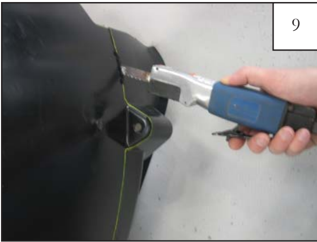
Using a metal hacksaw, pneumatic hand saw, or other suitable cutting device, trim the splash shield along the marked lines.
