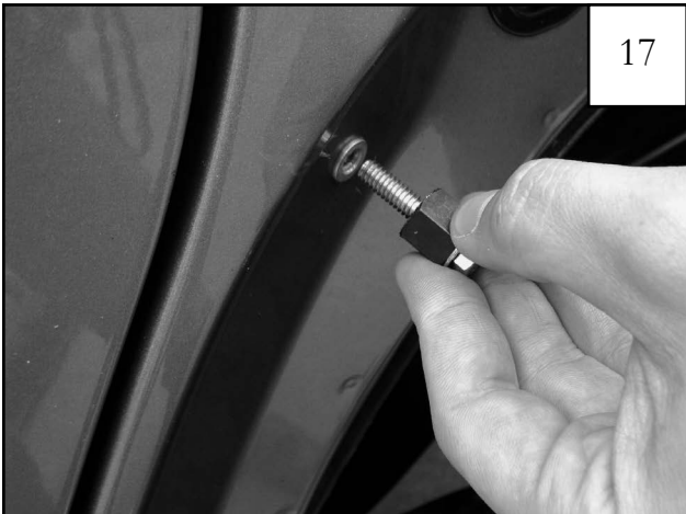
Remove rivnut tool. Repeat for remaining holes.
