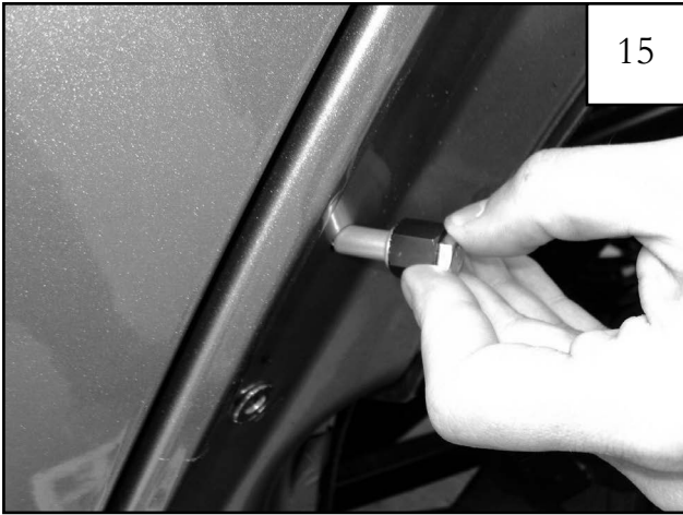
Insert rivnut in fender hole.
