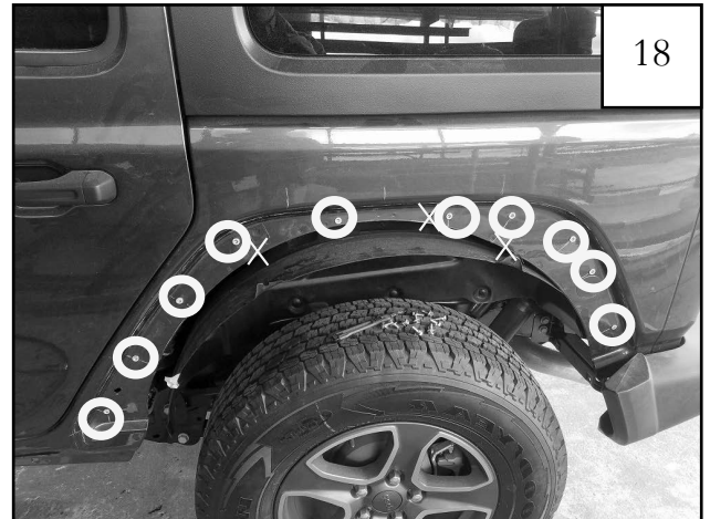
Install ten rivnuts in rear fender area using the same procedure as Steps 13 thru 17. Test fit inner pieces DR1, DR2, and DR3. NOTE: The "X" above indicates a hole that is not used.
