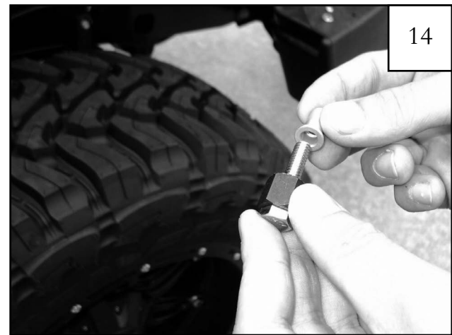
Place a rivnut on the provided rivnut tool.
