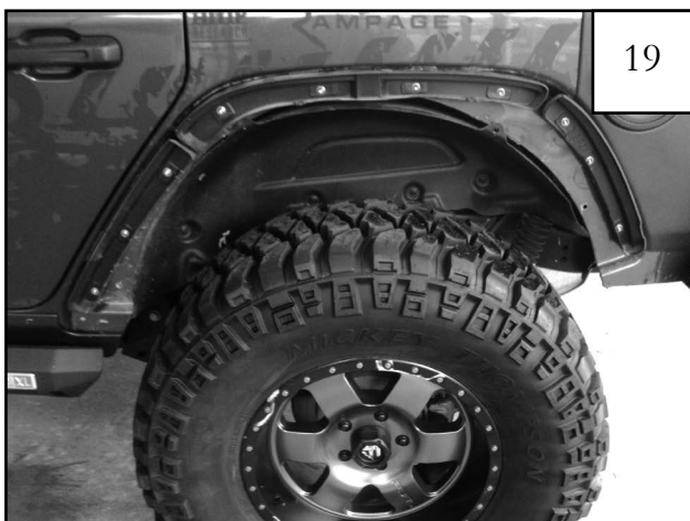
Slide a washer onto allen bolt. Insert a bolt/washer assembly through inner pieces and fender and secure to rivnut. Start the bolts but do not tighten.
