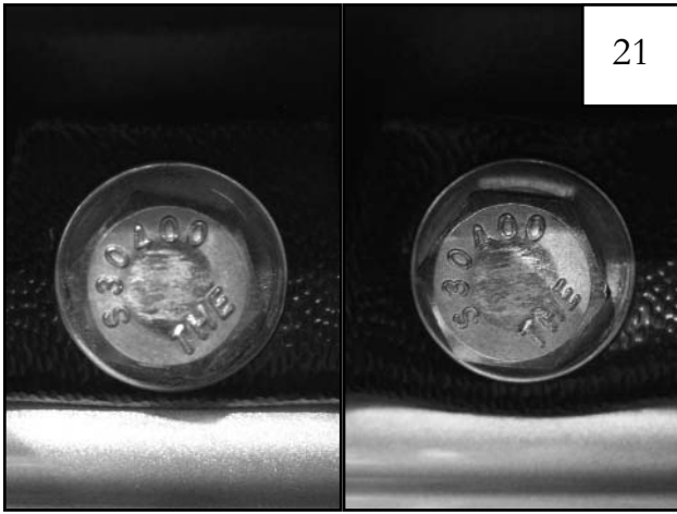
Bolt on left: Properly tightened; lower edge of inner piece runs straight Bolt on right: Overtightened; lower edge of inner piece bows down; if accidentally overtightened, remove inner piece completely before reinstalling
