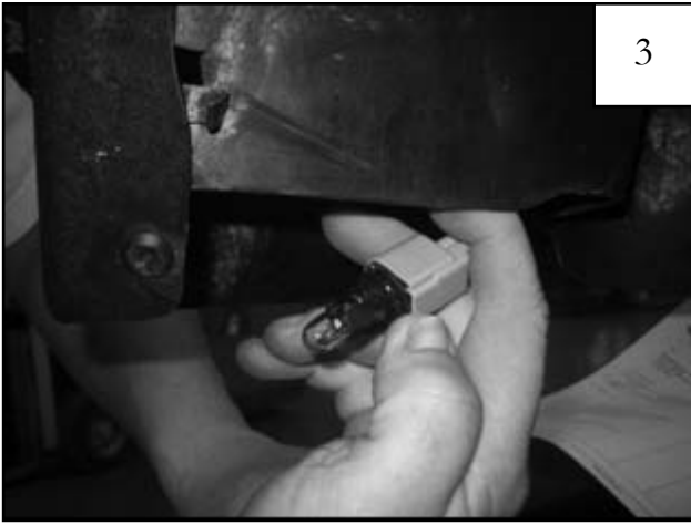
Remove light receptacle from light lens housing, letting it hang free of the housing.
