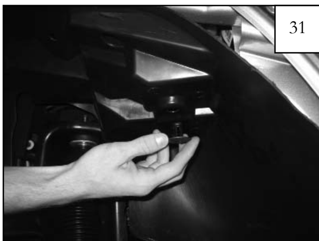
Reinstall factory fastener removed in Step 2 in location shown. 2007-2010 model years, fastener is a plastic thread engager. 2011-newer model years, fastener is a 10mm bolt.
