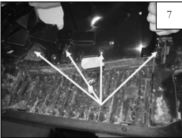
Use a pry tool or flat head screwdriver to remove four plastic fasteners.
