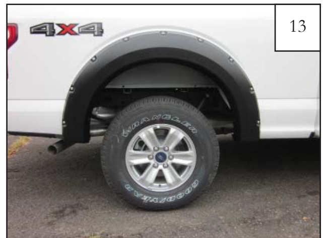
Completed rear flare installation.
