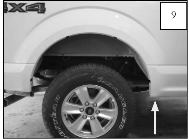
Install a supplied "S" clip (CL1-0005) over the mylar tab installed at the lower front of the rear wheel well.
