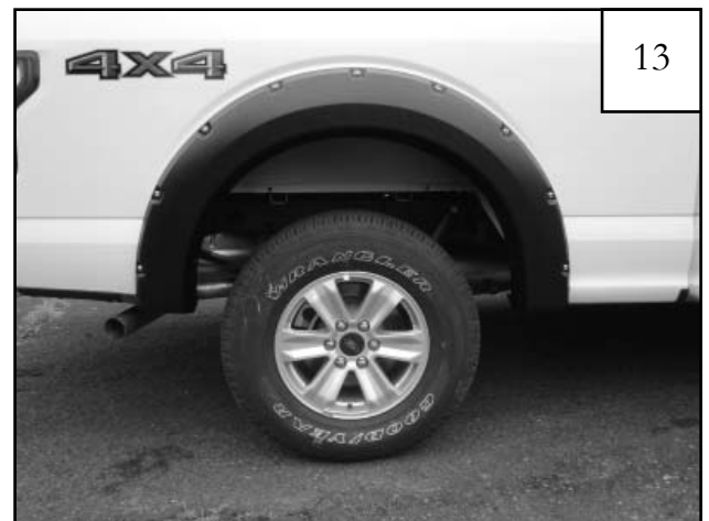
Completed rear flare installation.
