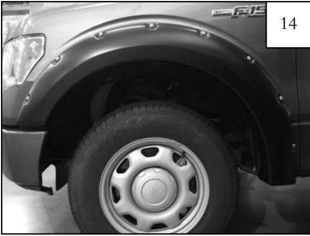
Completed front flare installation.
