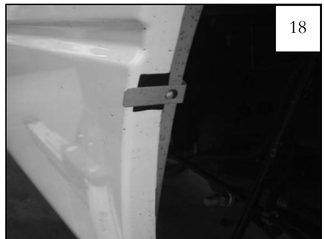
Install a Clip (CL1-0009) over each of the four Tabs (MT1-0014) placed on the sheet metal in Step 17.
