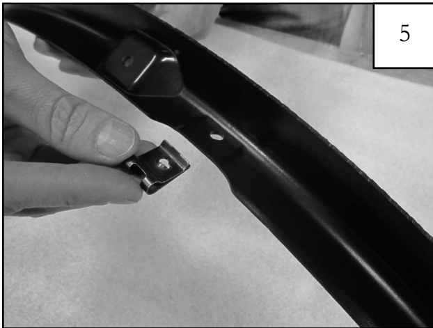
Verify presence of U-Clips on inner brackets.
