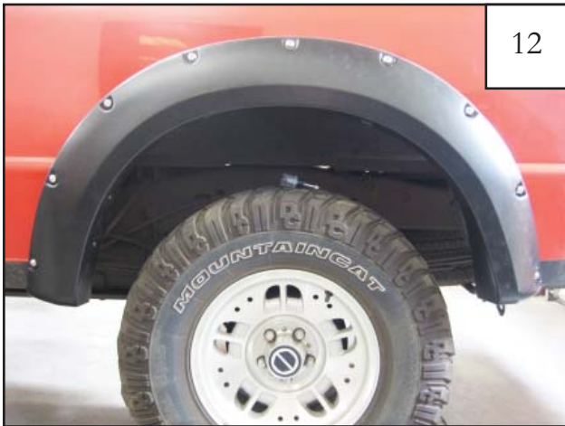
Completed rear flare installation.
