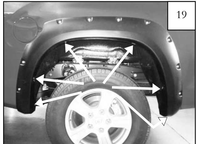
Hold flare firmly on the fender. Start a supplied Screw (SW1-0036) through each hole in flare and into hole in fender. (6 locations)
