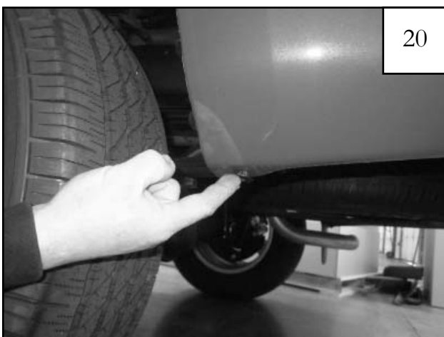
NOTE: If the lower rear wheel well does not contain a plastic grommet, insert supplied Grommet (GR1-0001) into the factory hole as shown.
