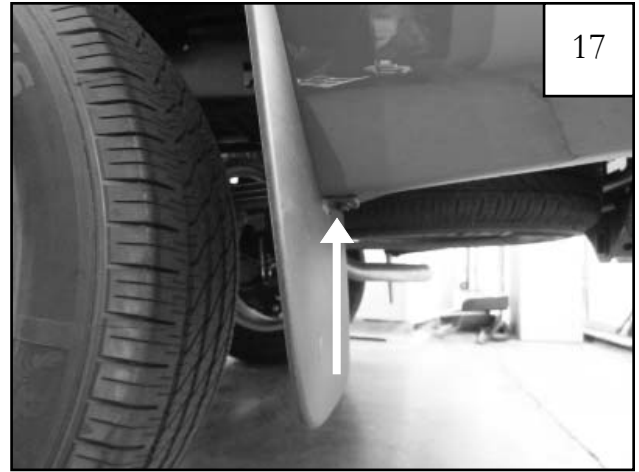
Remove one hex bolt from underside of mud flap using a 10mm socket. Discard mud flap.
