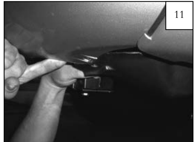
Pull down bumper cover and splash shield.
