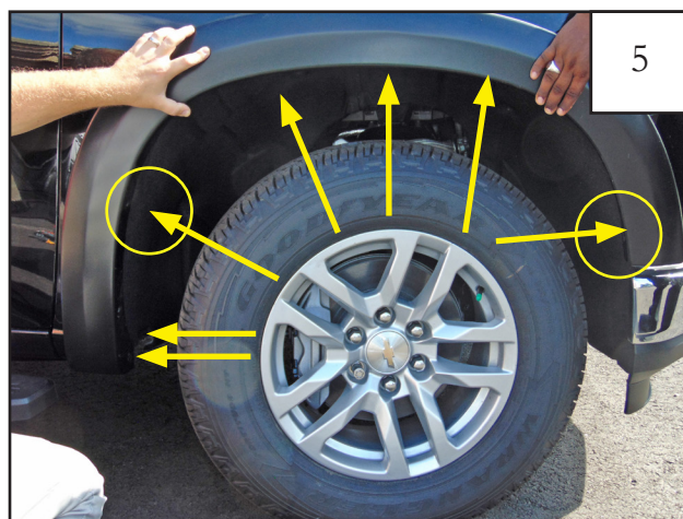
Hold flare to vehicle and note the approximate hole locations in the flare.
