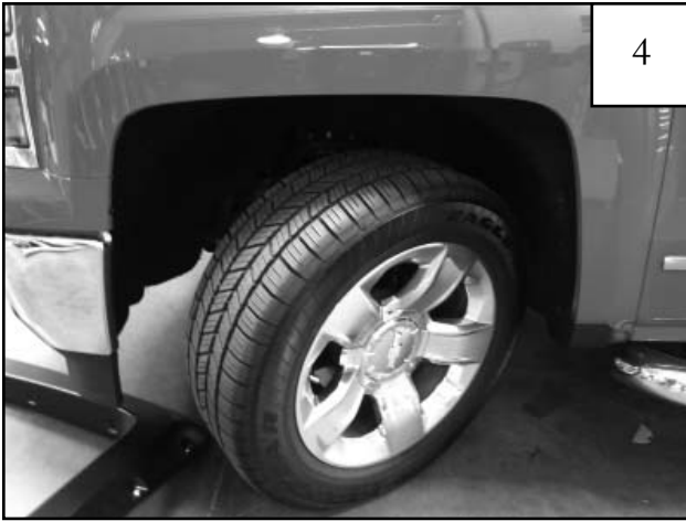
Turn front tire outward for easier installation.
