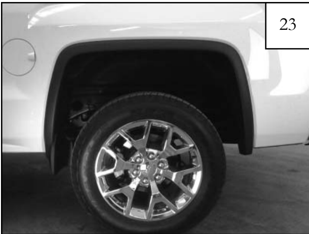
Factory wheel arch molding must be removed prior to part installation. See next steps.
