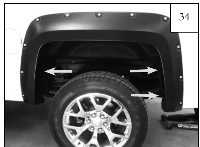
Hole locations to be marked for drilling.
