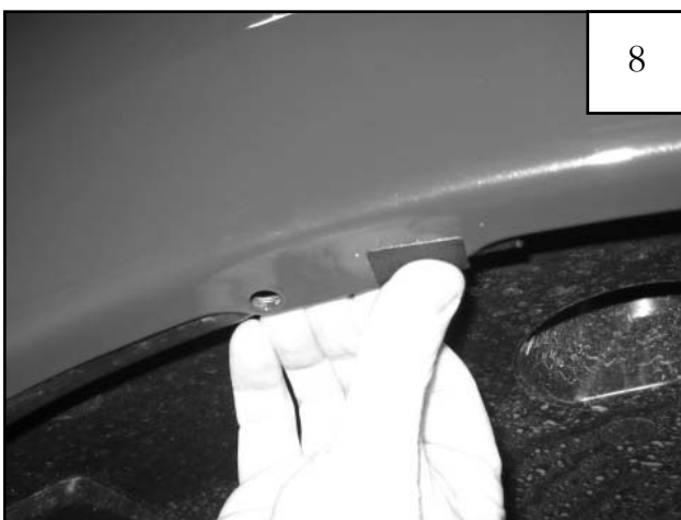
Install plastic tab over existing factory hole.
