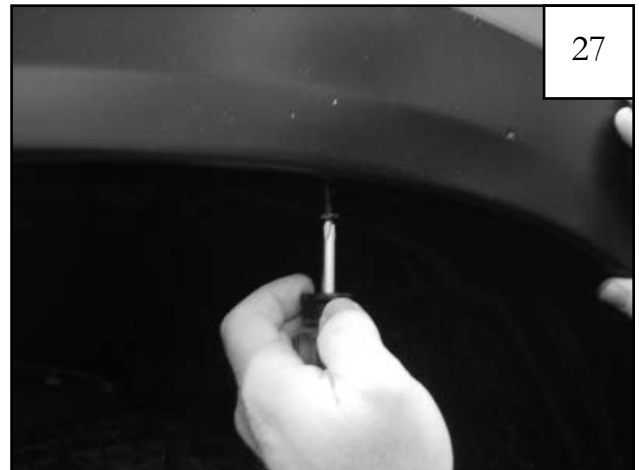
Start supplied screw (SW1-0056) using a Phillips screwdriver. Do not tighten. Pictured here is the top center screw location of the rear wheel well.
