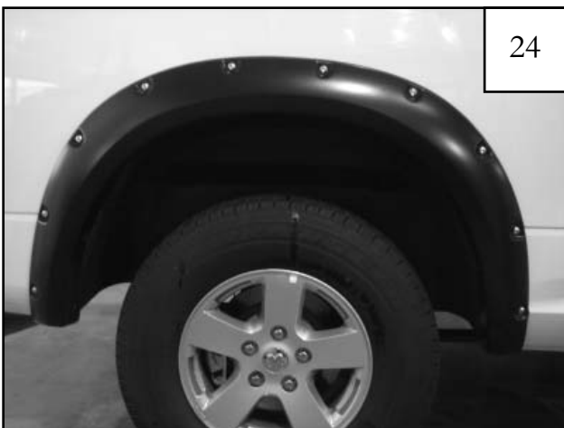
Completed rear flare installation.
