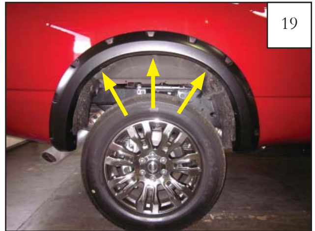
19 Position flare on rear fender and install 3 supplied screws (SW1-0058) through flare and into the clip holes.
