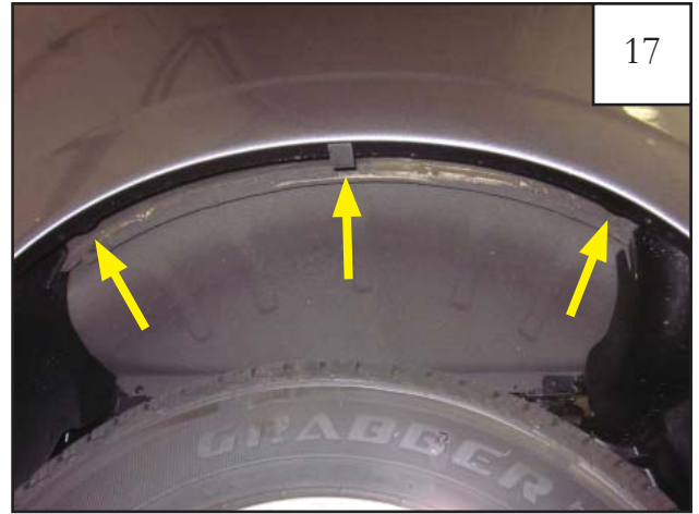
17 Install a foam tab (MT1-0034) over 3 top center metal tabs in the wheel well
