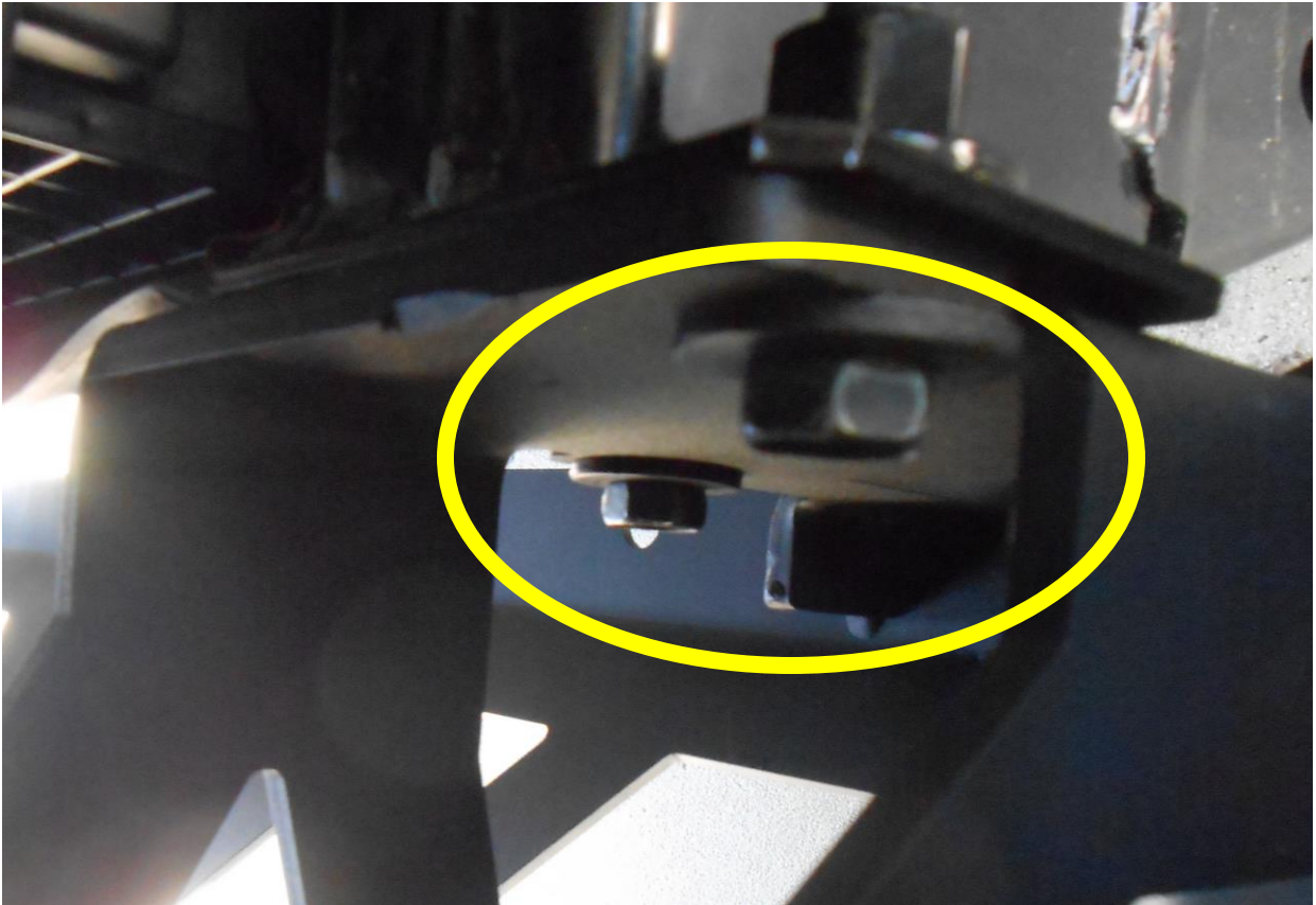
Figure 7b (bumper mounted to frame)
