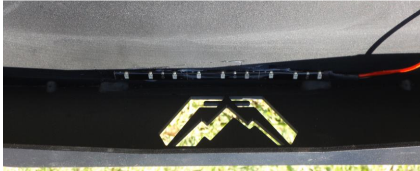
Figure 10 (light strip adhered to bottom of step)
