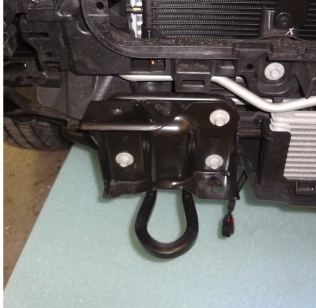
Figure 3b (TOW HOOK & OEM MOUNTING BRACKET)
