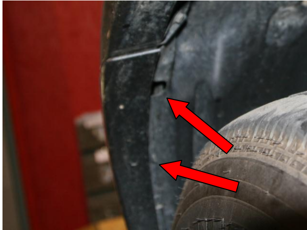
Figure 3 – Fenderwell fastener removal
