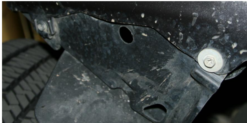
Figure 4 – OEM bumper cover screw removal
