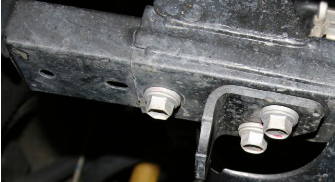
Figure 9 & 10 – Bumper beam extension and tow eye removal
