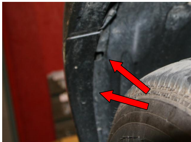
Figure 4 – Fenderwell fastener removal
