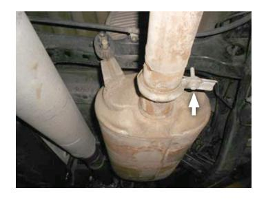
4. Unbolt bolts (x4) at both front flanged connections. Disassemble wire hangers from isolators then remove muffler assembly. Retain bolts for later use.
