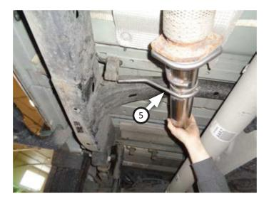
9. Place **clamp (7)** onto **muffler (2)** then connect it to inlet pipe. Tighten clamp just enough to allow for adjustment. Place (x2) **clamps (6)** onto muffler outlets.
