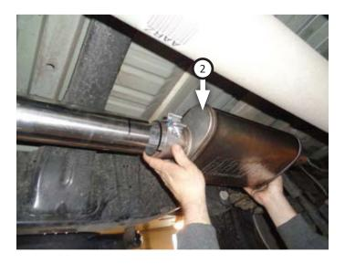
Transfer isolators from vehicle mounts to tailpipe assembly (3). Then route tailpipe assembly over rear axle and into muffler. Connect isolators to wire mounts and tighten clamps just enough to allow for adjustment.
