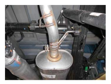
4. Remove and retain nuts (x2) on flanged connection behind catalytic converter. Separate hanger on pipe from isolator then lower assembly from vehicle.
