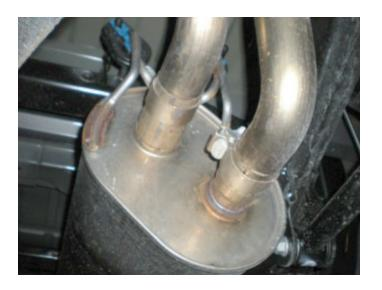
4. Loosen clamp on muffler inlet, then remove hangers (x2) at muffler rear from isolators. Slide muffler rearward to disconnect it from inlet pipe then lower and set it aside.
