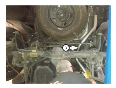
11. Remove isolator from factory mount (from step 4) and install it onto **left front tailpipe (4)**. Insert tailpipe wire hanger into factory mount then connect inlet to muffler. Tighten clamp just enough to allow for adjustment.
