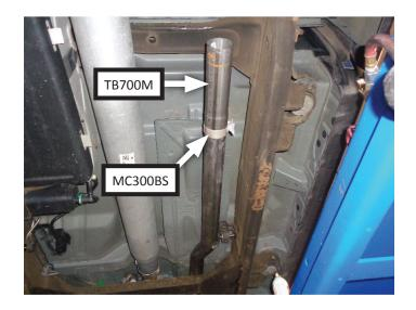
NOTE: Every slip fit connection in this kit must seat 3" deep except for the (x3) muffler connections which must seat 2" deep. Locate all components in your kit with a slip fit connection and mark them accordingly so your Flowmaster exhaust system fits properly onto your vehicle.
