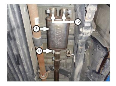
12. Fasten left frame hanger (10) to vehicle using bolt (16), backing plate (11), (x2) flat washers (18), lock washer (19) and nut (20). Then hang rubber hanger (15) on frame hanger end.
