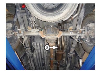
15. Place clamp (12) onto left rear tailpipe (6) and connect it to left overaxle pipe. Mount wire hanger into rubber hanger. Tighten clamp just enough to allow for adjustment.
