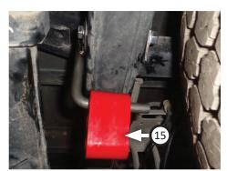
13. Route **right tailpipe (4)** over rear axle then connect it to passenger side muffler outlet. Insert wire hanger into stock mount to complete connection. Tighten clamp just enough to allow for adjustment.
