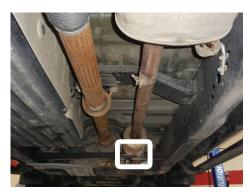
4. Disconnect factory muffler wire hangers (x2) from isolators on vehicle frame.
