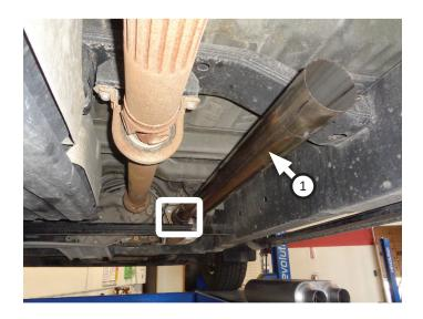
10. Place clamp (13) and front clamp hanger (9) onto extension pipe (2). Hang assembly onto vehicle frame and connect to inlet pipe.
