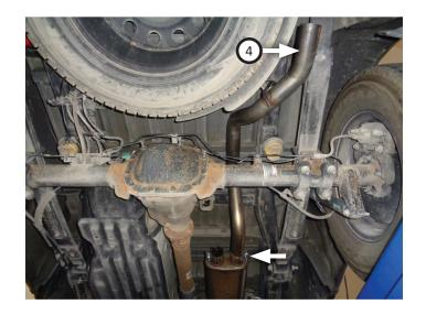
14. Route **left overaxle pipe (5)** over rear axle then connect it to driver side muffler outlet. Insert wire hanger into stock mount to complete connection. Tighten clamp just enough to allow for adjustment.
