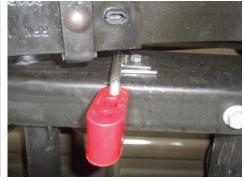
12. Route **left front (4)** and **right front (5) tailpipes** over axle then connect them to muffler. Insert their wire hangers into isolators and tighten clamps just to hold parts.
