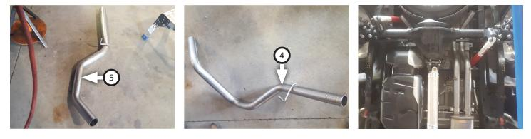
Place clamp (9) and mount (removed step 6) onto right rear tailpipe (7) then connect it to right front tailpipe. Bolt mount onto frame then tighten clamp enough to allow for adjustment.
