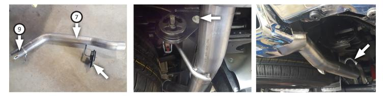
15. Place clamp (9) and mount (removed step 4) onto left rear tailpipe (6) then connect it to left front tailpipe. Bolt mount onto frame then tighten clamp enough to allow for adjustment.
