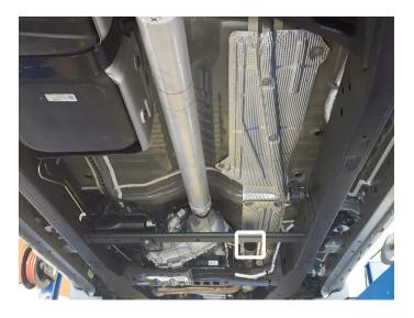
8. Release tab and remove factory clamp from pipe inlet. Retain factory clamp for later use.
