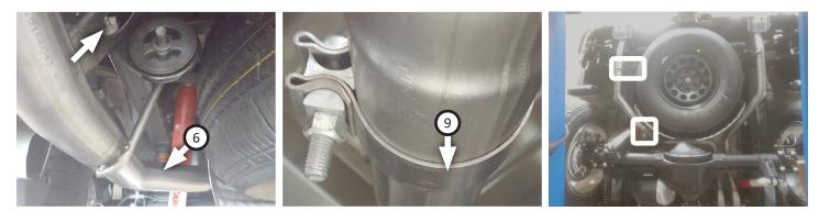
16. Adjust exhaust components for fit; maintaining ½" clearance and compensating for suspension, travel and vibration then tighten all clamps. Finally, fit (x5) hanger keepers (10) onto each sideways hanger.
