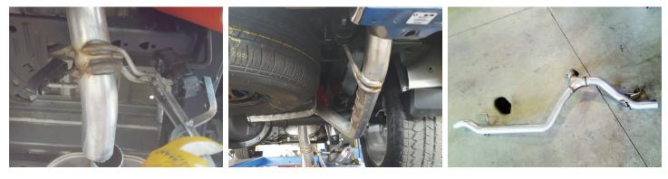
Loosen factory clamp from catalytic converter connection to disconnect inlet pipe, disassemble wire hanger from isolator then remove muffler assembly completely from vehicle.
