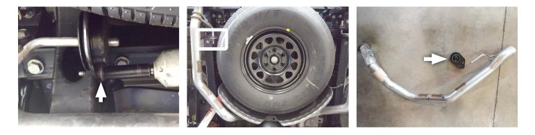
5. Cut tailpipes just behind factory muffler.
