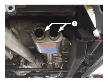
Route right front tailpipe (5) and left front tailpipe (4) over axle and connect them to muffler outlets. Mount wire hangers into isolators then tighten clamps (x2) enough to allow for adjustment.
