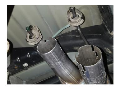
12. Place (x2) **clamps (9)** onto direct fit muffler outlets then connect factory tailpipes to them. Adjust muffler and exhaust system until it is oriented correctly then tighten all clamps just enough for later adjustment.
