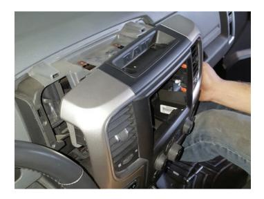
16. Unplug connector plug for 12V DC socket in lower left corner of console.
