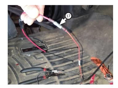
20. Place wire tap (18) onto fuse holder then close them around blue socket wire. Pinch fuse holder to splice fuse wire in with socket wire, then close fuse holder to encase connection.
