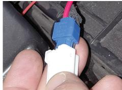
21. Open fuse holder cap, plug in **micro fuse (16)**, then replace cap.
