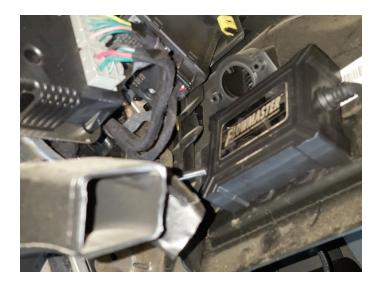
24. Find accessory point (behind battery on driver side), cut slit or x in it and insert a coat hanger wire through into cab. Attach control unit connector to wire, apply lubricant to it then draw it into engine compartment.
