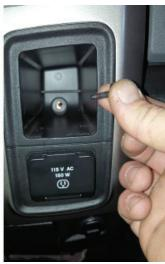
15. Pull center console front off of dashboard just enough to gain access behind it. Leave all wiring attached.
