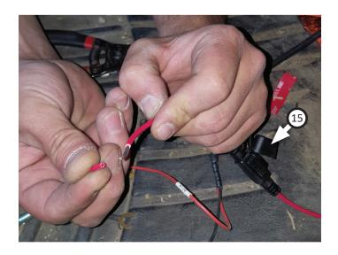
19. Insert stripped ends of fuse holder and control unit into **butt connector (17)**. Crimp connection, then apply heat to middle of butt connector to seal wires together.
