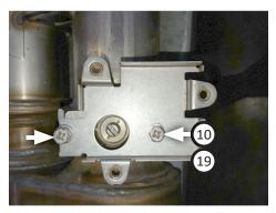
8. Set **valve spring (4)** into place on muffler valve underneath actuator mount assembly.
