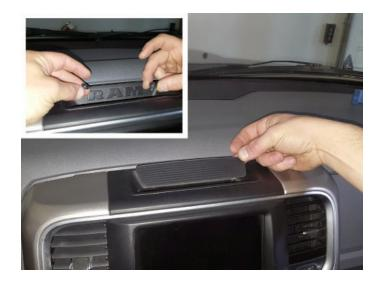
14. Remove console center compartment cover and fastener; retain them for later use.
