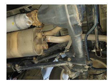
4. Loosen clamp at front of muffler, unclip ground wire and disassemble muffler from mounts. Remove muffler from vehicle, making sure isolators stay attached.
