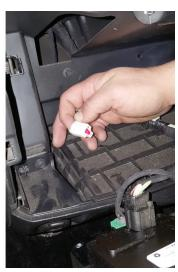
17. Remove or trim 12V DC socket wire wrap until you have enough wire to splice into.
