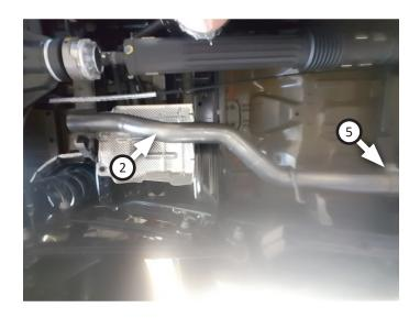
9. Place clamp (5) onto tailpipe assembly (3) and route it over axle then connect it to mid pipe. Re-bolt rear hanger mount back onto vehicle and tighten clamp just enough to allow for adjustment.
