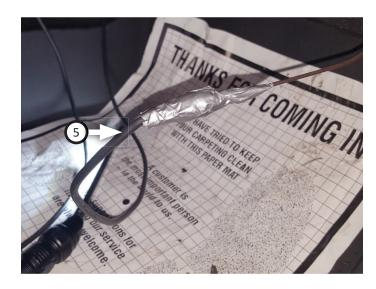
14. Cover connection with lubricant then pull it back through accessory point.
