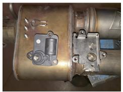
8. Place valve spring (3) into groove in muffler outlet then fasten actuator motor (4) onto mount ensuring valve spring lines up properly. Secure parts using (x3) bolt assemblies (8).
