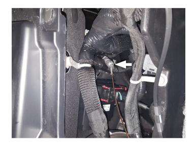
15. Remove wire, tape and lubricant from controller kit end. Pull wire assembly up and connect ends together. Secure any slack away from moving and heated engine components.
