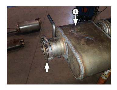
7. Place fiber spacer (18) onto actuator mount assembly (2), then fasten them onto muffler with (x2 ea.) fiber washers (17) and bolt assemblies (8).
