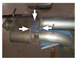
Fasten muffler flange to factory flange using (x2) bolts (9), (x4) flat washers (10), (x2) lock washers (11) and (x2) nuts (13). Secure rear of muffler to exhaust using clamp (7). Re-connect grounding wire.
