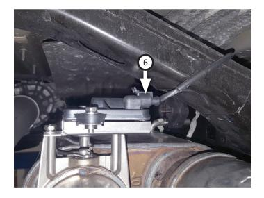
**NOTE:** You may secure wire assembly several different ways; **zip tie (14)** it to factory wire bundle, tuck it behind heat shield, secure it to frame, etc. Just be sure that connections are stable and wire is protected from heat.
