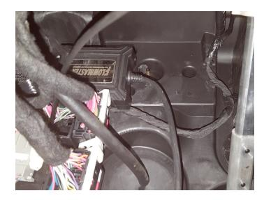
17. Strip end of controller kit red wire. Connect **fused circuit** tap (16) to it then crimp connection.
