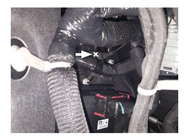
13. Thread hanger wire into cab through accessory point from last step. Then bend wire and connect it to controller kit end. Tape over connection to secure it.
