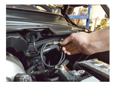
16. Open underside of dashboard under driver side. Fasten controller kit to a point up and away from interfering with vehicle operation.
