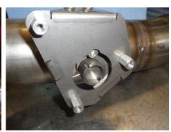
Insert screws (x3) (10) through actuator and flat washers (x3) (11). Place actuator onto tailpipe valve mount then tighten screws to fasten assembly. Complete step for both tailpipe assemblies. CAUTION: Make sure you place flat washer between actuator and standoff as shown, **NOT** beside screw head. Also, make sure the actuator spring is properly aligned between actuator and valve.
