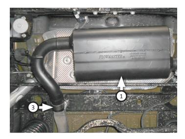
817437 Rev 09/23/19  Place clamp (3) onto muffler outlet then connect tailpipe assembly (2) to it. Insert wire hanger into rubber hanger then tighten clamp just enough to allow for later adjustment.
