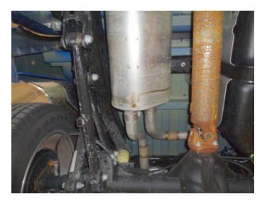
4. Support muffler with a stand, remove muffer wire hangers from isolators then loosen ring clamp at muffler inlet connection. Slide muffler off of front pipe and set aside.
