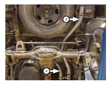
At rear of frame on driver side of vehicle (next to spare tire), is a pair of attached hanger mounts. Place rubber hanger (11) onto inner hanger.
