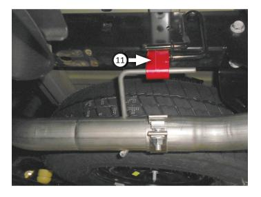
12. Place clamp (9) onto left rear tailpipe (5) and connect it to left front tailpipe. Set wire hanger at rear of tailpipe into rubber hanger, then tighten clamp just enough to allow for adjustment.
