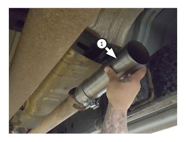
Place clamp (10) onto AMT muffler (2) then connect it to adapter pipe. Tighten clamp enough to allow for adjustment then place clamps (x2) (9) onto muffler outlets.
