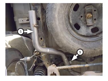
**NOTE:** This kit includes both side and rear exit pipes. A side exit is preferable for towing purposes, to avoid blowing fumes in or on vehicles you may be towing (eg: RV trailer, boat, etc). Otherwise, if you wish to equip your vehicle with a rear exit exhaust, use **rear exit pipes (6)** now in place of side exit pipes.
