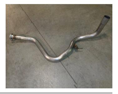
Remove bolts (x4) at both front flanged connections. Disassemble wire hangers from isolators and remove muffler assembly. Retain bolts for later use.
