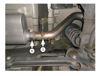
9. Place clamp (6) onto exit pipe (4) then connect it to over-axle pipe. Insert wire hanger into isolator then tighten clamp just enough to hold parts.
