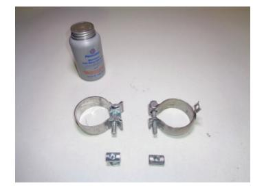
6. Mark 2" reference lines on cut factory pipes for muffler install. Install (x2) clamps (2) on muffler (1) inlets.
