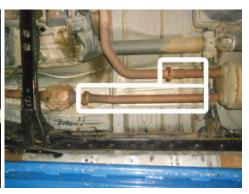
4. Remove bolt and clamp from muffler outlet, dismount wire hangers (x3) from mounts and remove factory muffler from vehicle. Dismount factory tailpipe from mounts and remove from vehicle.
