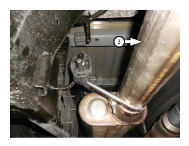
9. Place clamp (14) onto muffler (4) inlet then connect it to extension pipe. Tighten clamp just enough to allow for adjustment then place clamps (x2) (15) onto muffler outlets.
