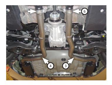
9. Replace ground strap (removed step 4) onto hanger on right tailpipe.
