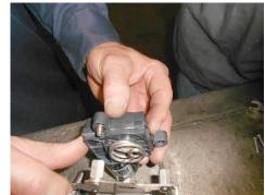
10. Complete step on both actuators and tailpipes: Ensure center arm of actuator spring sets between top and bottom mount tabs, then tighten (x3) screws securely.
