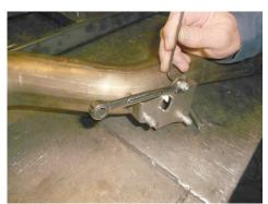
9. Complete step on both actuators and tailpipes: Place actuator on mount, with spring oriented between tabs then loosely attach it using (x3 ea.) screw (10) and flat washer (12).
