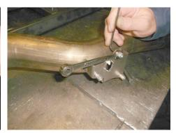
8. Complete step on both actuators and tailpipes: Place actuator on mount, with spring oriented between tabs then loosely attach it using (x3 ea.) screw (10) and flat washer (12).
