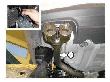
16. Recommended: Secure slip-fit connections with a 1-inch tack weld then spray high-temp paint over each weld to prevent rust and premature corrosion.
