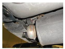
4. Remove (x3) nuts securing actuator to mounts then remove actuator and spring from mount on each tailpipe.
