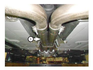
12. Place (x2) clamps (6) onto both muffler (4) inlets then connect them to scavenger pipe, sliding them 1¾" deep. Level mufflers and tighten clamps just enough to hold parts but still allow for adjustment.
