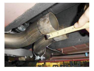
Place (x2) clamps (6) onto both muffler (4) inlets then connect them to scavenger pipe, sliding them 1<sup>1</sup>/<sub>4</sub>" deep. Level mufflers and tighten clamps just enough to hold parts but still allow for adjustment.
