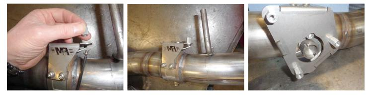
Place (x3) screws (10) into actuator and through (x3) flat washers (11). Fasten assembly to mount on tailpipe, aligning actuator spring into slot on mount before tightening fasteners. Repeat step on remaining tailpipe.
