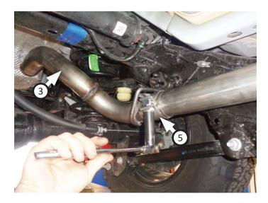
11. Place **clamp (5)** onto tailpipe, then connect it to over-axle pipe. Make sure tailpipe bend curves over suspension components, ensure connections are completely seated and tighten clamp.
