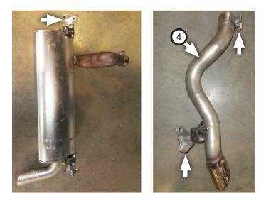
6. Remove stock resonator assembly from rubber isolator with a pry bar and retain for later re-use.
