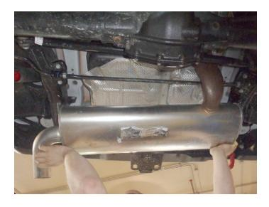
5. Transfer driver side mount and clamp from factory muffler to **tailpipe (4)**.
