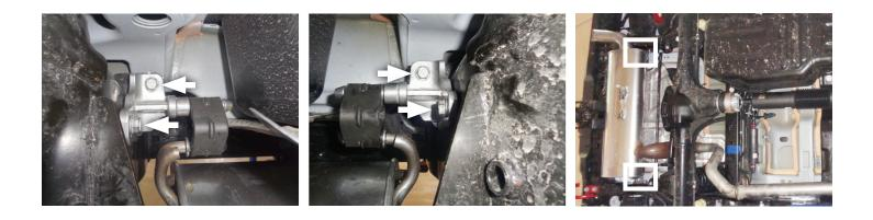
4. Loosen clamp at muffler inlet connection above rear axle then remove muffler from vehicle.
