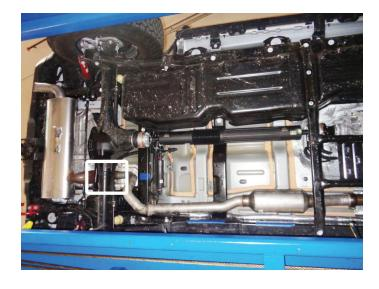
5. Place stock muffler next to **muffler (4)** oriented in the same direction. Then transfer driver and passenger side mounts over.
