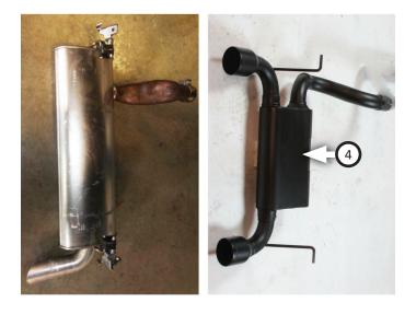
6. Remove wire hanger on resonator assembly from isolator, and loosen bolt on clamp at resonator inlet.
