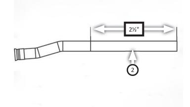
Place factory clamp (removed step 8) over outlet of factory pipe, connect **resonator (1)** to factory pipe, then tighten clamp enough to allow for adjustment.
