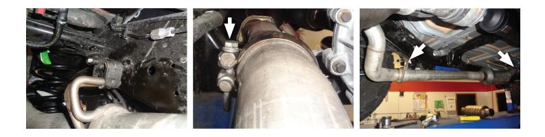
7. Remove resonator assembly from vehicle and retain clamp for re-use.
