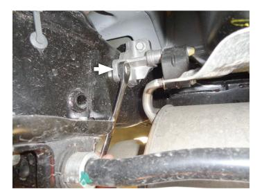
4. Remove upper bolt from left and right rear mounts, disassemble hangers from isolators and remove muffler from inlet pipe. Transfer driver side hanger mount onto new tailpipe.
