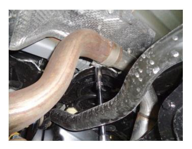
4. Remove left and right rear mounts supporting muffler. Then with an assistant, slide muffler off of inlet pipe and remove it from vehicle and transfer mounts over to corresponding sides of American Thunder muffler.
